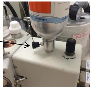
26. Press **sputter**, if it doesn't sputter press reset. The current should be 10mA- adjust the voltage dial on the electronics box if needed. If the plasma flickers, open the needle valve until stable. The plasma should be a blue, if consistently pink ask a member of bioimaging staff. May be prep chamber has warmed up or the vacuum needs checking.
