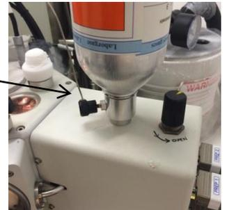
27. Press **sputter**, if it doesn't sputter press reset. The current should be 10mA- adjust the voltage dial on the electronics box if needed.
