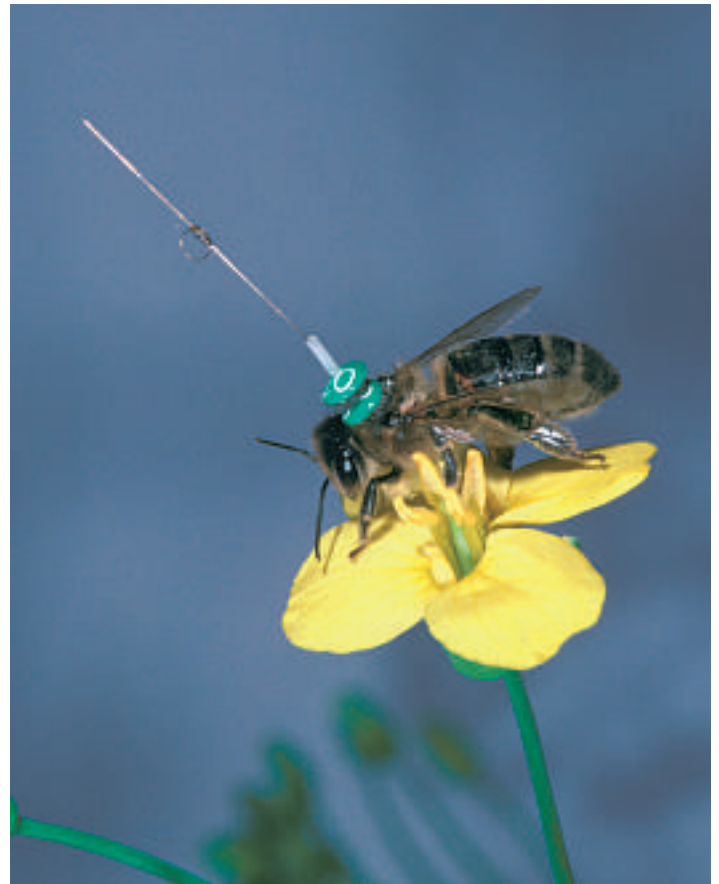
Figure 2: A honeybee fitted with a transponder. The transponder, which does not need a battery to operate, can be detected by the Rothamsted scanning harmonic radar at a range of just under 1 km. The combination of transponder and radar allows records of insect flight trajectories over hundreds of metres to be made.
