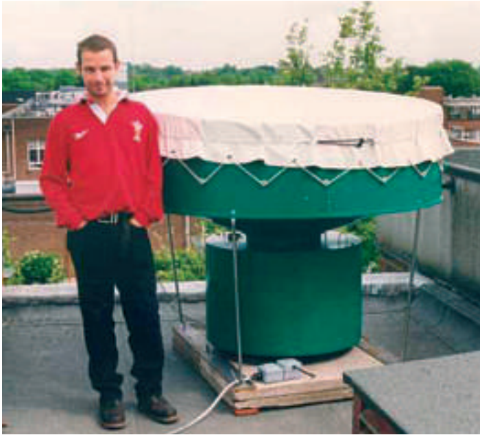
Figure 1: A vertical-looking radar installed at Rothamsted Research. The radar is controlled by a personal computer, and operates 24 hours a day throughout the year, monitoring the passage of overflying insects in the altitude range from approximately 150m to 1200m above ground level.
